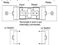
Use Relays and Switches that have high contact reli-Note: ability because the current flowing from terminals 1 or 3 is as small as approx. 10 µA. OMRON's G3TA-IA/ID is recommended as the SSR.
